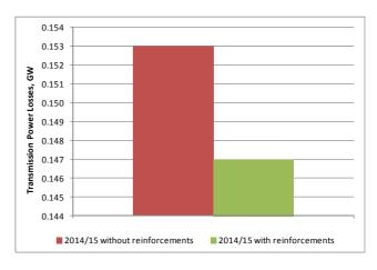
Figure 1: Impact of Reinforcement Projects on Transmission Losses at Peak Demand with 'Gone Green' scenario
