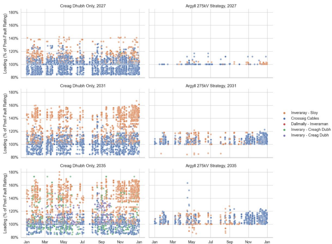
Figure 20 Intact and contingency network loading violations for the Leading the Way local scenario
