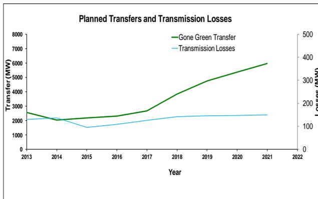
Figure 1: SHE Transmission Planned Transfers vs Transmission Losses
