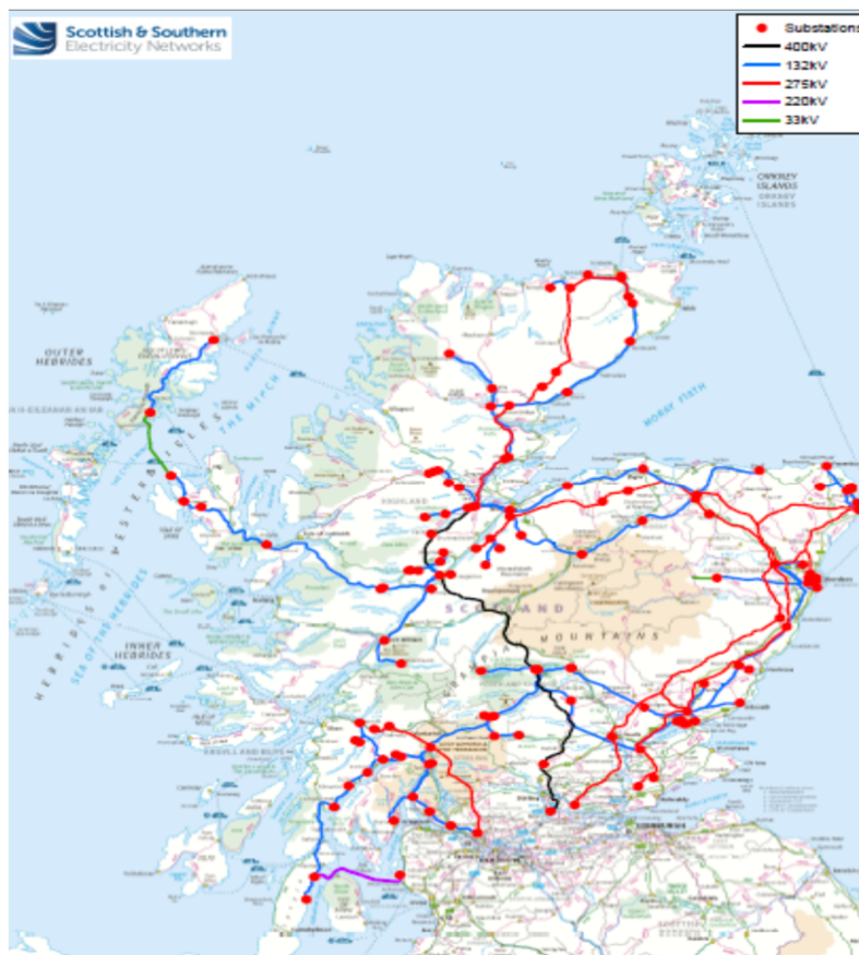
Figure 3 – Existing Transmission System
