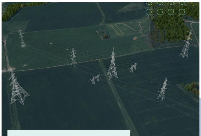
When crossing transmission lines the initial preference is to have the two lines cross over each other in what is called a diamond arrangement. Each design would be specific to the individual crossing however an illustration is provided below of this option. The avoids the use of underground cable and minimises the land sterilisation caused by cable sealing end compounds.
