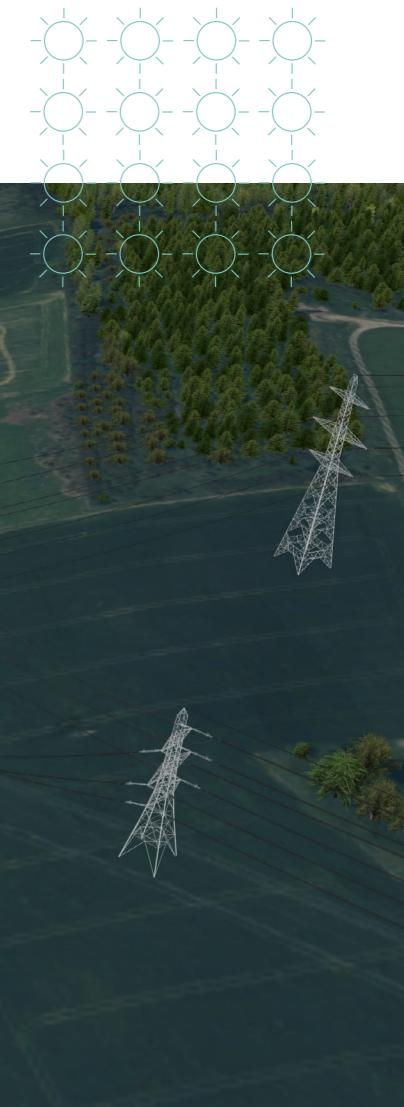
The design of the towers ensures that the lowest point to ground beneath the wires is at a minimum **9m** in all locations under normal operating conditions.
