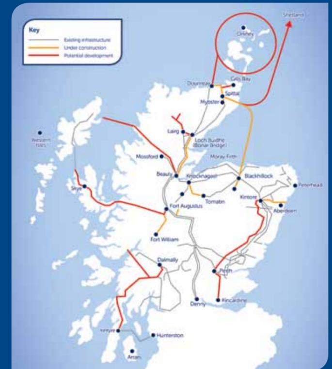
In total we maintain about 5,000km of overhead lines and underground cables – easily enough to stretch across the Atlantic from John O’Groats all the way to Boston in the USA.
