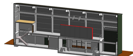
Long section through cable basement
