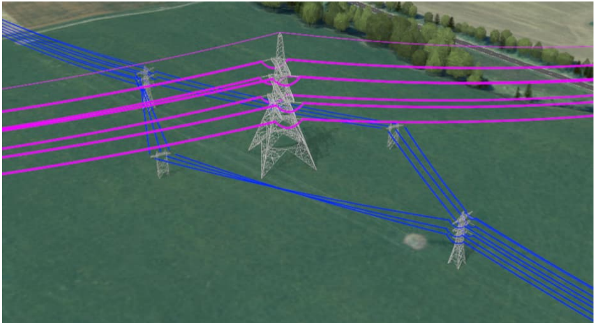
Plate 3.1a: Diamond Crossing Example (Pink OHL is proposed 400 kV OHL; blue is existing OHL)
