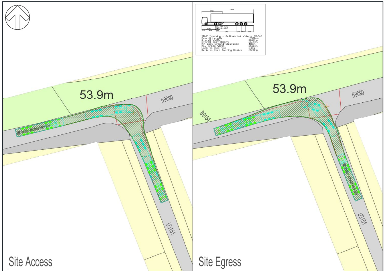
Figure 13.1.7.27: Potential Constraint at B9090 / U3151 Junction
