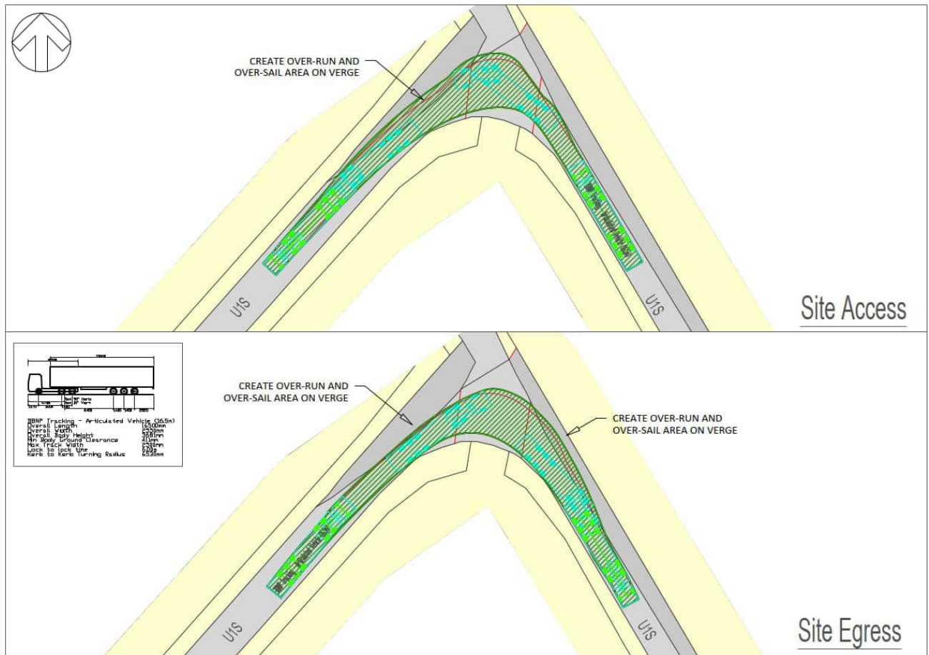
Figure 13.3.7.34: Potential Constraint at Bend on U1S
