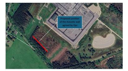
An acoustic fence will be installed in the location shown to increase attenuation lost during the storm in 2024 (attenuation loss due to fallen trees). Installation in Winter 25/26.
