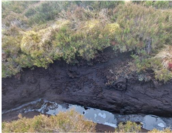
Insert 2 - Photograph of peat exposure within a drainage ditch in northeast of main works area taken during site reconnaissance in March 2024
