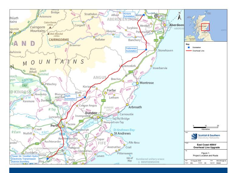
The OHL upgrade works would involve replacing the conductors, insulators and fittings on the existing overhead line steel lattice towers between Kintore, Fetteresso, Alyth (future substation) up to the border with Scottish Power Transmission (SPT) near to Blairingone (east of Stirling). SPT will carry out similar works on their section of the OHL. This will allow the overhead lines to operate at 400kV.
