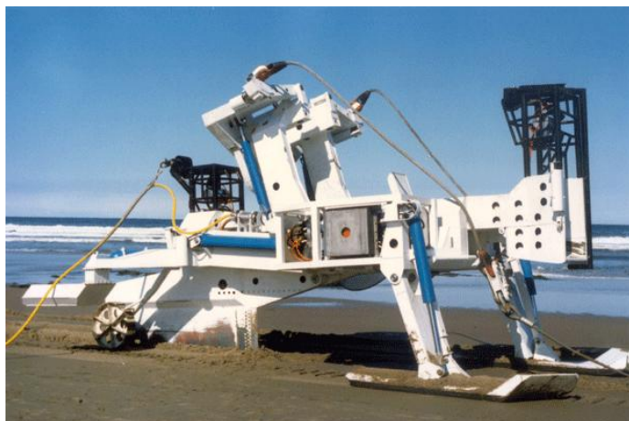
Figure 3-10: Example of a typical cable plough
