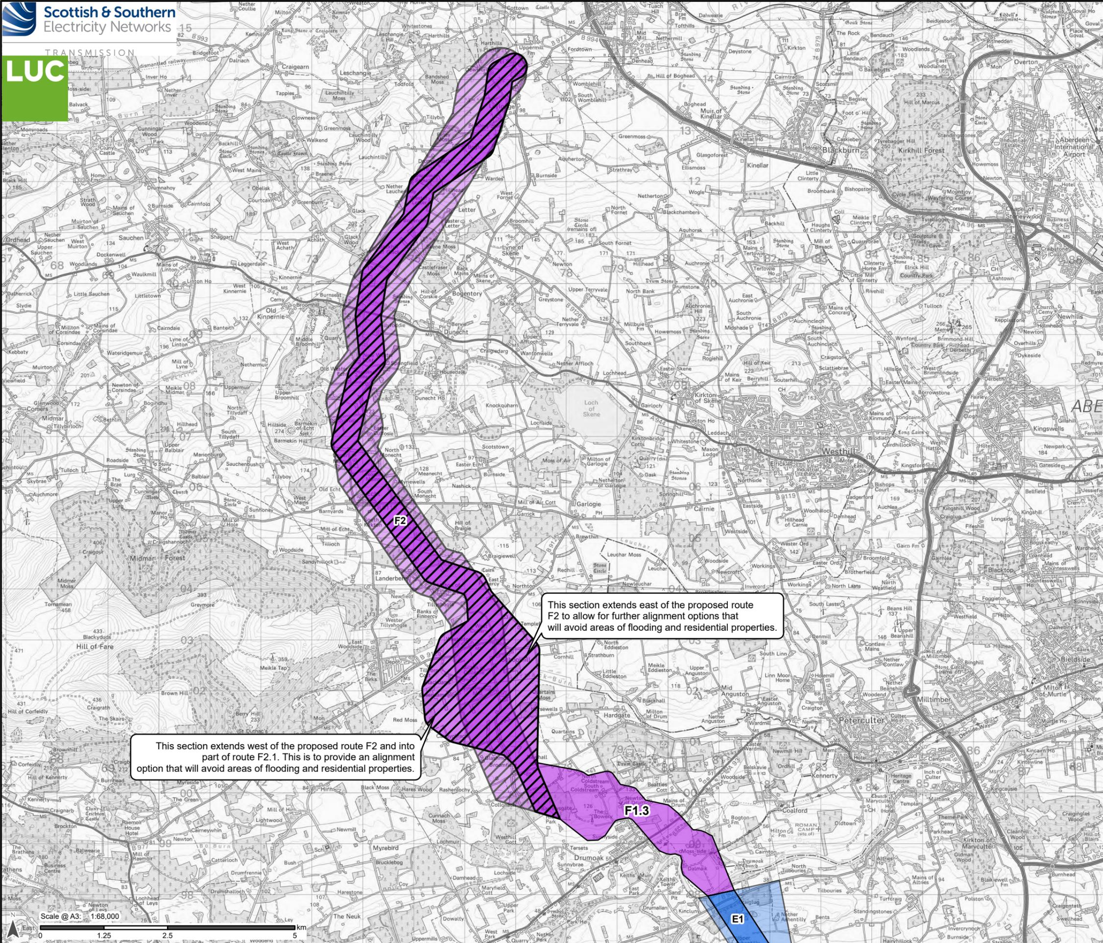
This section extends west of the proposed route F2 and into part of route F2.1. This is to provide an alignment option that will avoid areas of flooding and residential properties.
