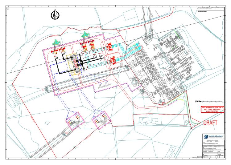
This design is an example of the scale of footprint and equipment used within a potential GIS substation design at Kintore, this is not a final design solution.
