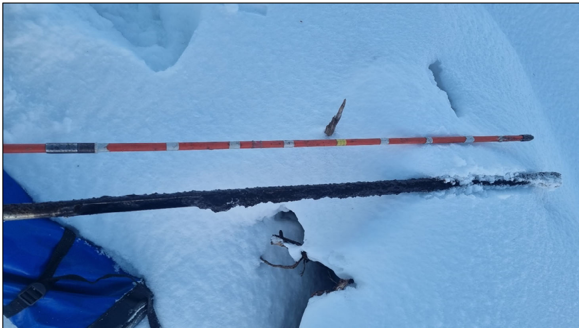
Photo 13.1.3: Peat core (ID 11) taken near Tower N77 (Section E)
