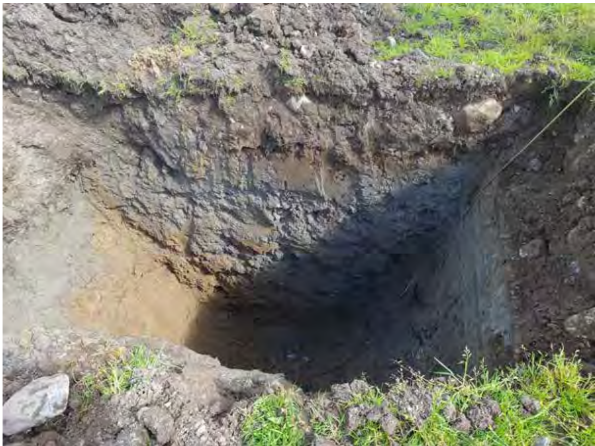
Plate 91 West-facing section of TP70 - c. 3m deep - clearly showing possible cut of mill pond
