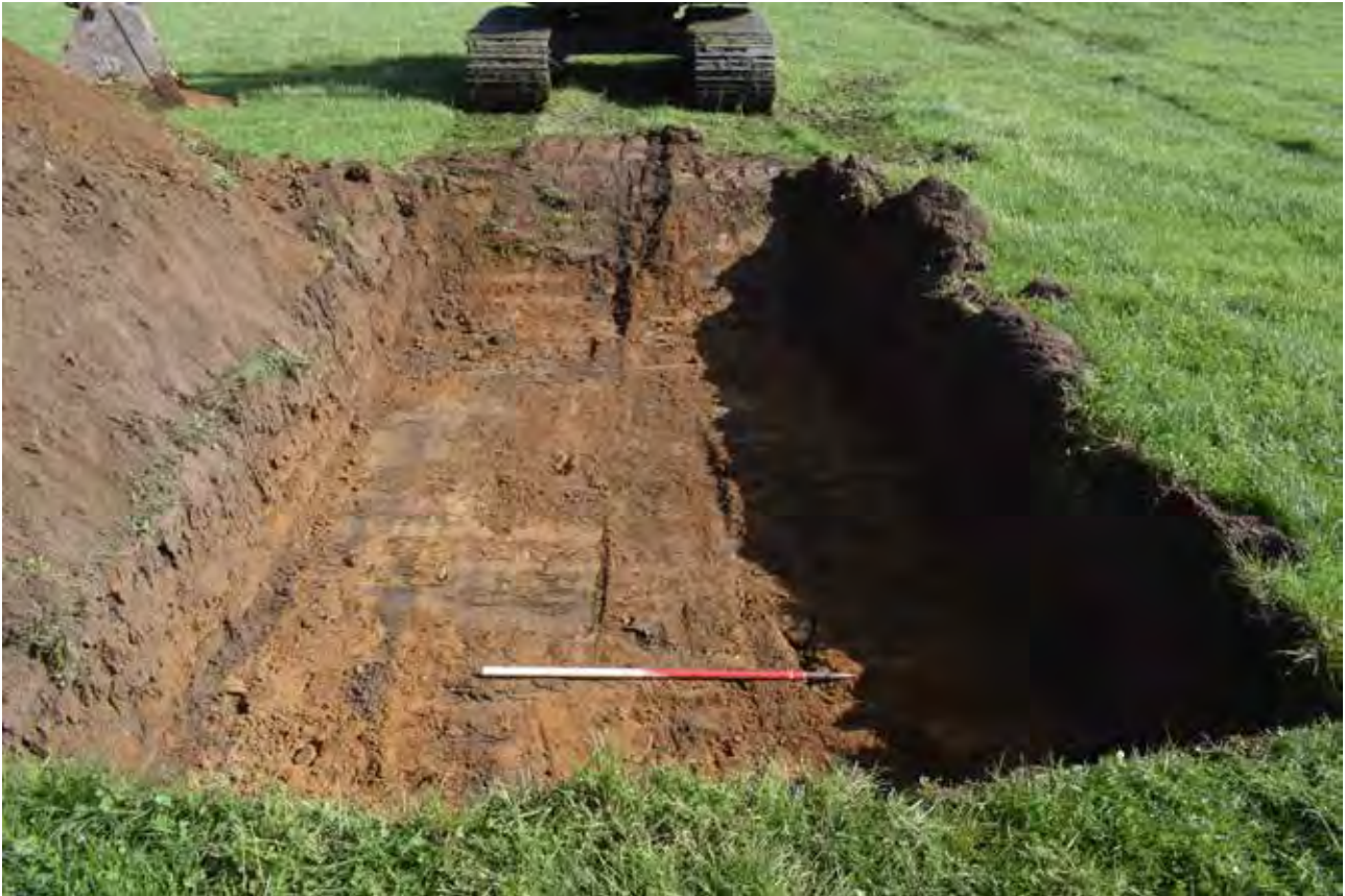
Plate 24 Post-excavation of TP16 extended for plate load test
