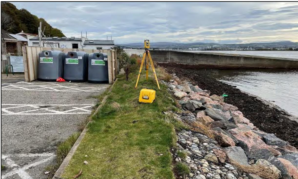
FIGURE 4 - S5 TOTAL STATION SETUP
