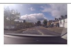
The AIL makes its way south through Beauly town centre. Parking restrictions will need to be put in place to prevent on street parking. There are speed control table tops and humps in the road which it is assumed the load can negotiate. This will need to be confirmed by the specialist haulage company.
