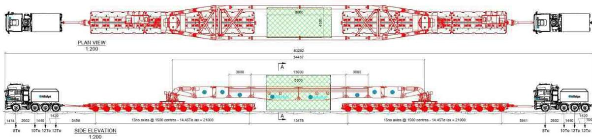
Figure 2 275 te transformer loaded onto 30-axle Girder Frame Trailer
