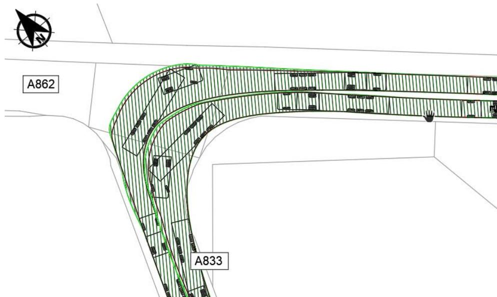
Figure 6.7 HGVs entering / exiting the A833 junction with the A862 eastbound
