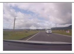
There are numerous services passing over the A9 carriageway. The overhead lines appear to have more than sufficient clearance to allow the AIL to pass under them, however, targeted survey will be required to confirm this.
