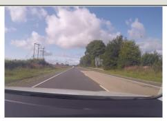
The AIL enters the A9 heading south towards Alness. The A9 is of a high geometric standard. Numerous services pass overhead but these appear to have suitable clearance ,however, targeted survey will be required to confirm this. The AIL will require the full width of the carriageway cross section.
