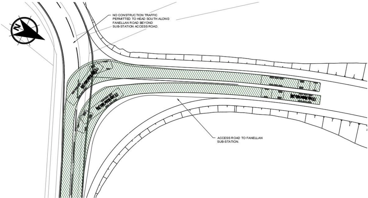
Figure 6.5 HGVs entering / existing C1106 / sub-station access road junction
