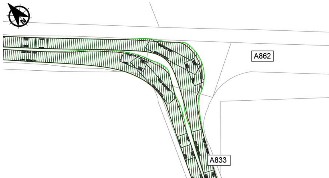
Figure 6.6 HGVs entering / exiting the A833 junction with the A862 westbound
