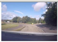
The AIL is required to enter the Nigg Roundabout in an anti-clockwise direction. The diagram 610 nonilluminated bollards located on the deflection island at the B9175 will be required to be removed and replaced and the load will over run the deflection island. The AIL enters the A9 on the northbound carriageway, towards oncoming traffic. Some localised widening of the carriageway is required in both the inner and outer circumference of the roundabout to allow the load to pass.
