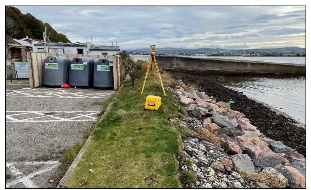
FIGURE 4 - S5 TOTAL STATION SETUP
