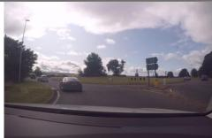
The entrance to Tore Roundabout is wide enough to allow the load to enter the roundabout. The load will be required to pass through part of the centre of the roundabout... A temporary running surface will be required through the area of central roundabout island. No modification will be required at the entries or exists to the roundabout which would be more complex. See drawing 65209842-SWE-XX-XX-D-H-0016 for the extents of the improvement required.
