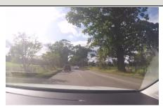
The AIL heads south on the A862 heading towards Beauly. The road is of a good standard with cross section in the region of 7.0m. The AIL will take the full cross section of the road. Large sections of the route are tree lined which may require localised trimming so not to damage the transformer unit.
