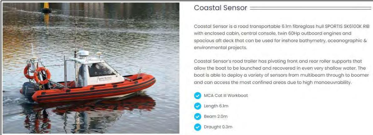
FIGURE 6 - SURVEY VESSEL COASTAL SENSOR
