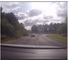
The AIL will require the full cross section of the carriageway to access the A9 (southbound). To enter the A9, the load will need to pass on to the northbound A9 off slip carriageway. The first non-illuminated deflection bollard will need to be removed and reinstated to allow the load to pass through.
