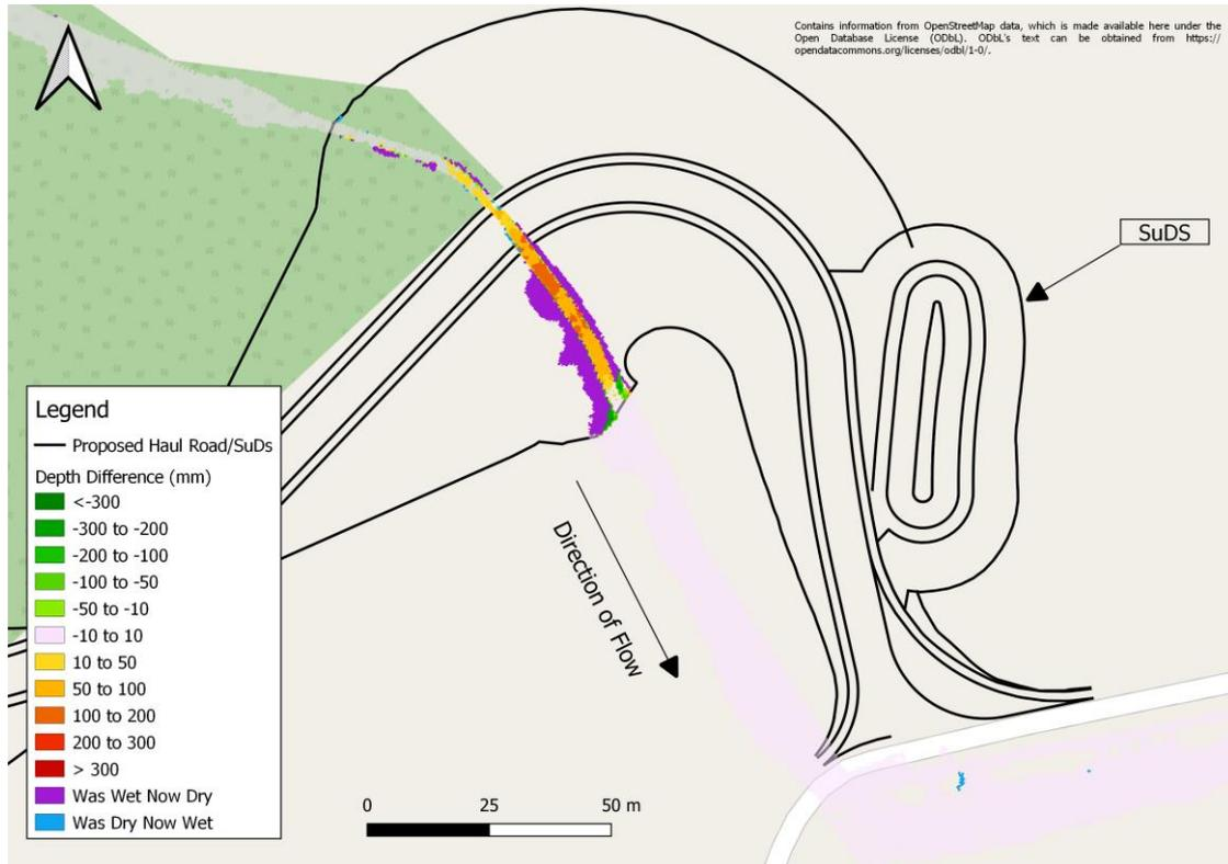
Figure 4-5. Proposed vs Baseline Depth difference and wet/dry change.
