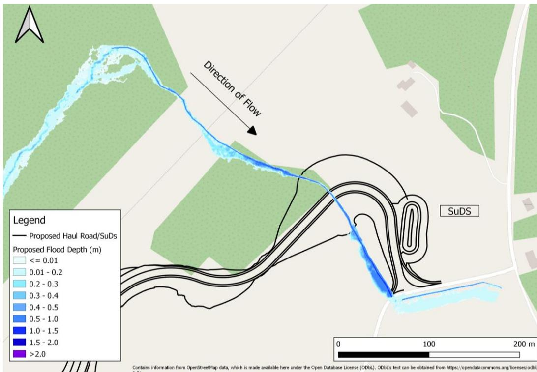
Figure 4-4. Proposed 0.5%AEP +CC flood extents.
