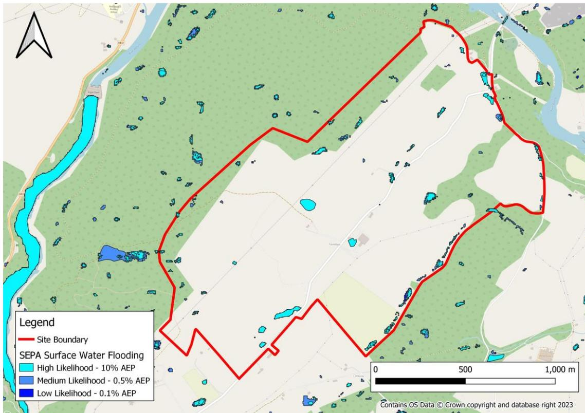
Figure 4-6: Extract from SEPA Surface Water Flood mapping.
