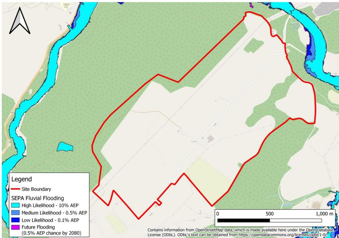
Figure 4-1. Extract from SEPA Fluvial Flood mapping.
