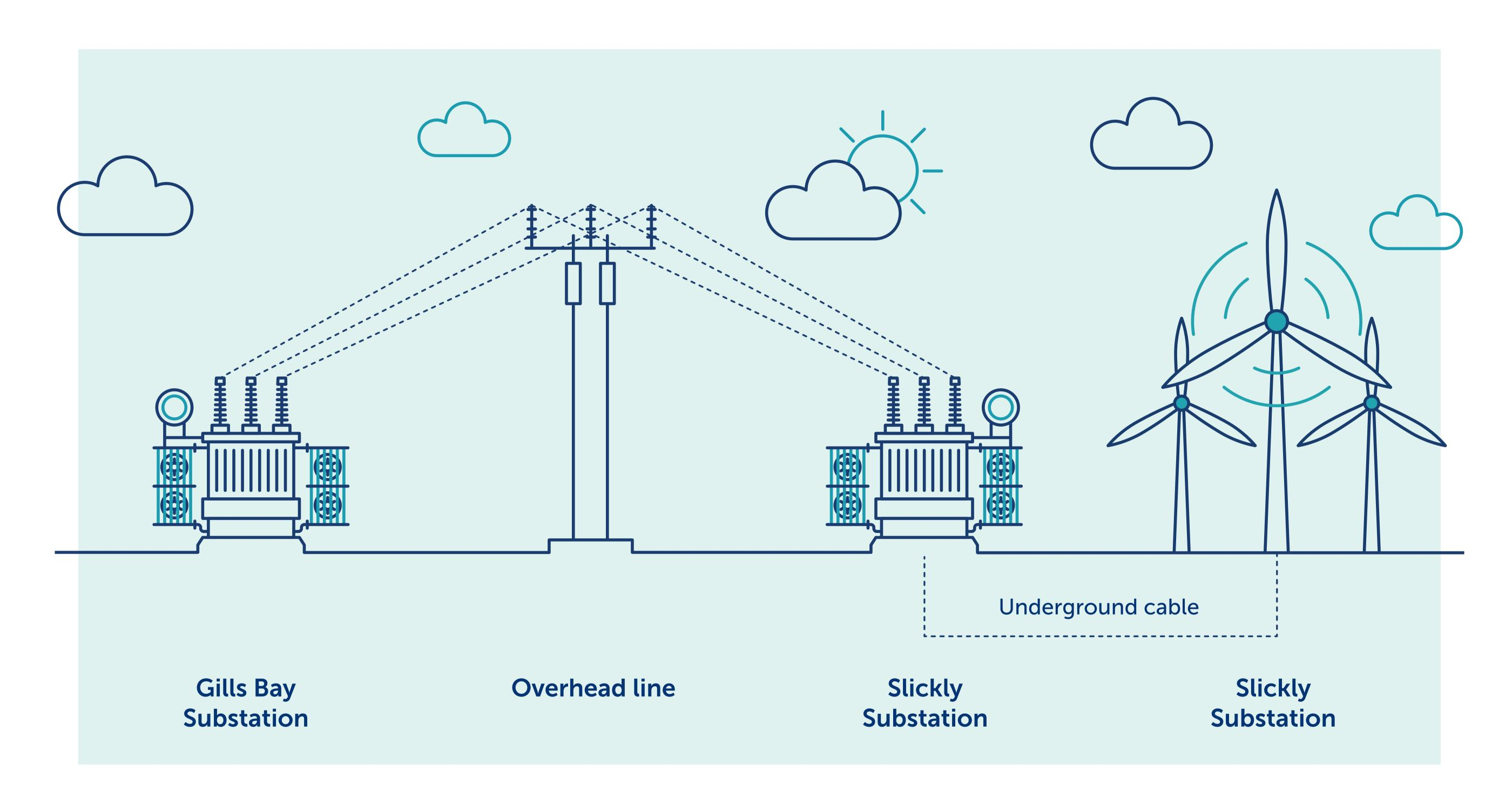
The connection comprises a single circuit 132kV trident wood H pole arrangement, as shown, supporting the overhead line running a distance of approximately 8.5km in length between the proposed Slickly wind farm substation and the Gills Bay substation (being proposed and constructed under a separate SSEN-T project).
