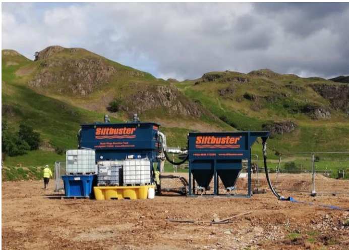
Figure 24: Example of flocculant dosing system from Siltbuster
