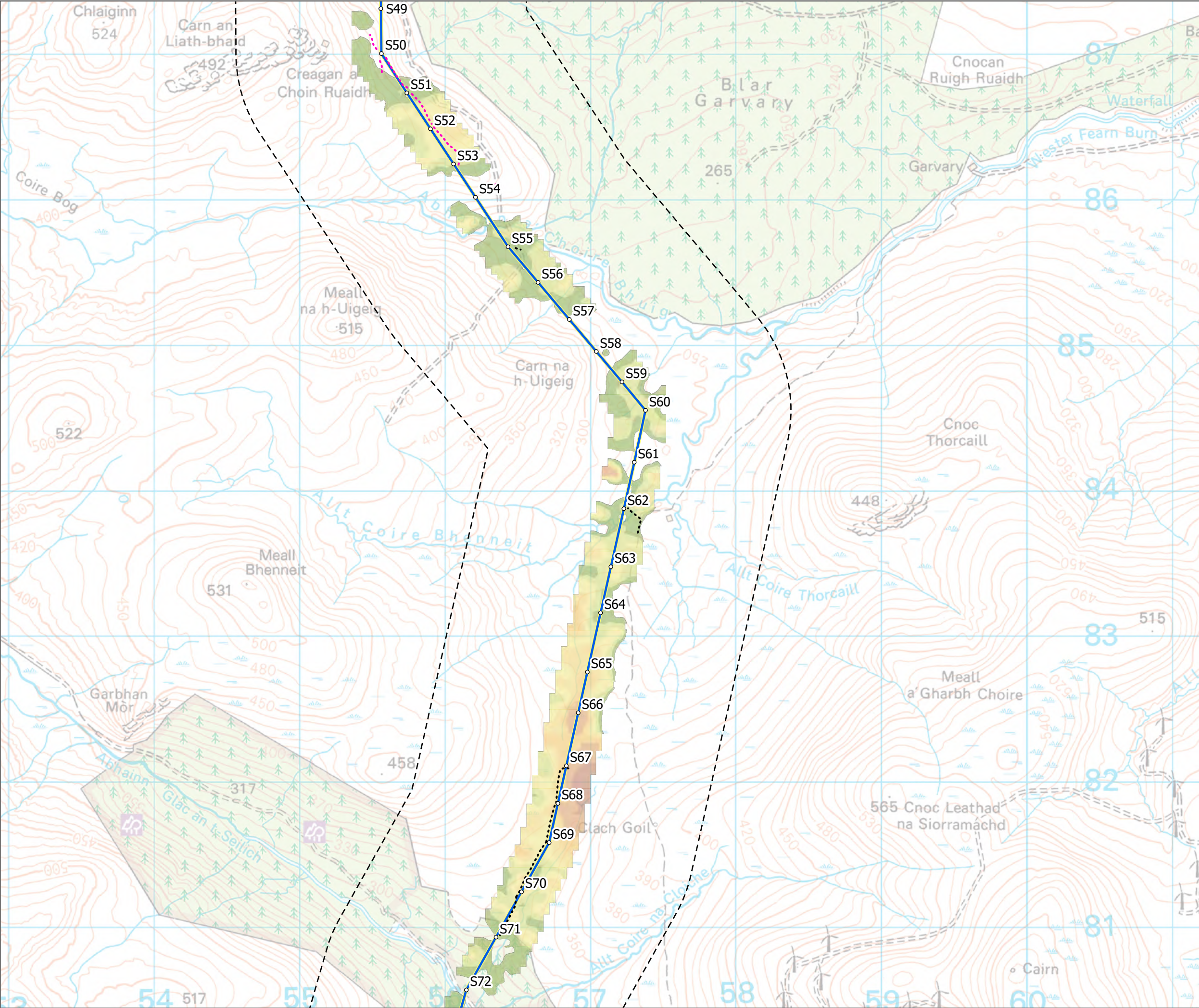
Figure 8 - 21 Spittal - Loch Buidhe - Beaully 400 kV OHL Connection Peat Landslide Hazard Risk Assessment Floating Tracks (PLHRA)
