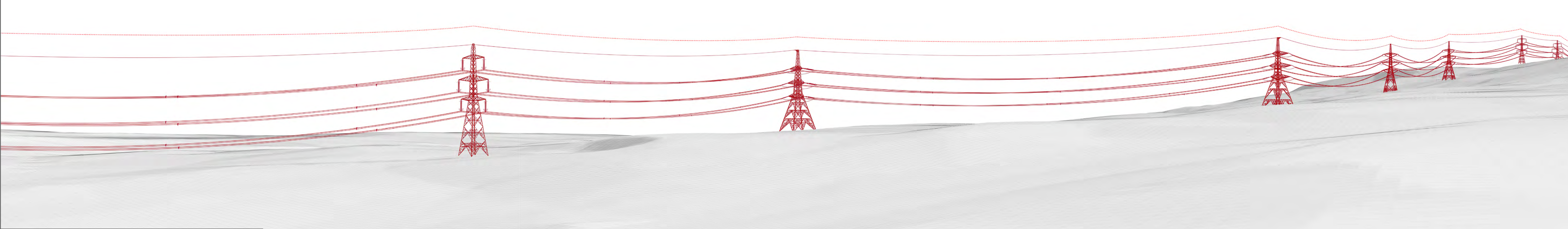
Wireline Drawing - Proposed Development Shown In Red ----- Vertical Limit of Deviation: the maximum height of a tower above ground level
