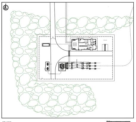
The indicative substation layout view set out opposite provides an example of a current, typical single grid, transformer substation (outdoor arrangement footprint circa 50m x 80m). At each of the four sites, similar arrangements will be designed in order to suit the site specific functional requirements and land restrictions.
