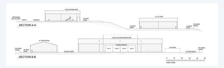
The subsea and underground cable at the heart of SSEN Transmission's proposals would use a technology called High Voltage Direct Current (HVDC). This is different to the existing island electricity network, which carries high voltage electricity as Alternating Current (AC). The HVDC Converter Station (a large substation-type installation) is required to convert AC electricity to HVDC, and vice versa, to connect the subsea cable to the Island's electricity network.
