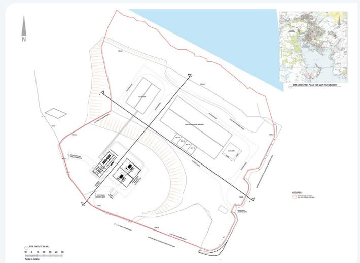
smaller buildings also required on the site, including an associated 132kV Gas Insulated Switchgear (GIS) substation. The proposed rating of the transmission link would result in a maximum building height of around 20m.
