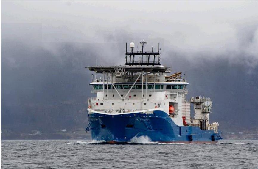
NKT Victoria CLV (cable lay vessel) used to lay HVDC subsea cable
